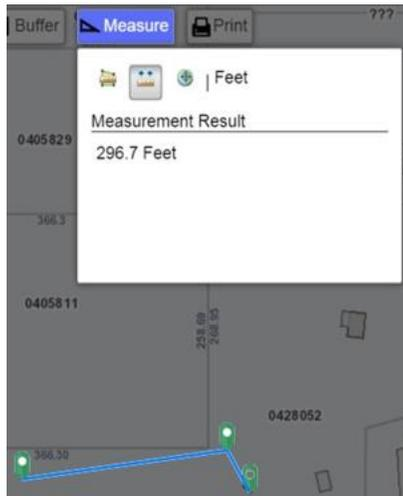
To use the distance measurement tool, select the second icon on the top of the measure tool. You can then begin drawing a line on the map.
